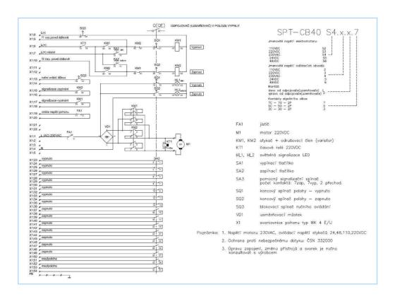
M1 - motor; KM1, KM2 - contactor + suppression component; FA1 - breaker; KT1 - time relay; HL1, HL2 - LED indicators; SA1 – breaking button; SA2 – making button; SA3 – auxiliary indication switch with 7 making, 7 breaking and 2 changeover contacts; SQ1 - limit switch to indicate the OFF position; SQ2 - limit switch to indicate the ON position; SQ3 - manual control blocking switch; VD1 - rectifier block; X1 - WK 4 E/U terminal board
