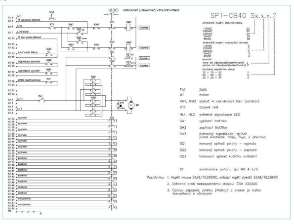
M1 – motor; KM1, KM2 – contactor + suppression component; FA1 – breaker; KT1 – time relay; HL1, HL2 – LED indicators; SA1 – breaking button; SA2 – making button; SA3 – auxiliary indication switch with 7 making, 7 breaking and 2 changeover contacts; SQ1 – limit switch to indicate the OFF position; SQ2 – limit switch to indicate the ON position; SQ3 – manual control blocking switch; VD1 – rectifier block; X1 – WK 4 E/U terminal board
